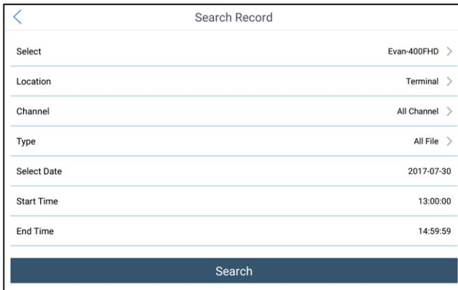
3. Enter the search conditions and tap the Search button, the recording files of selected vehicle will be displayed on the screen.
